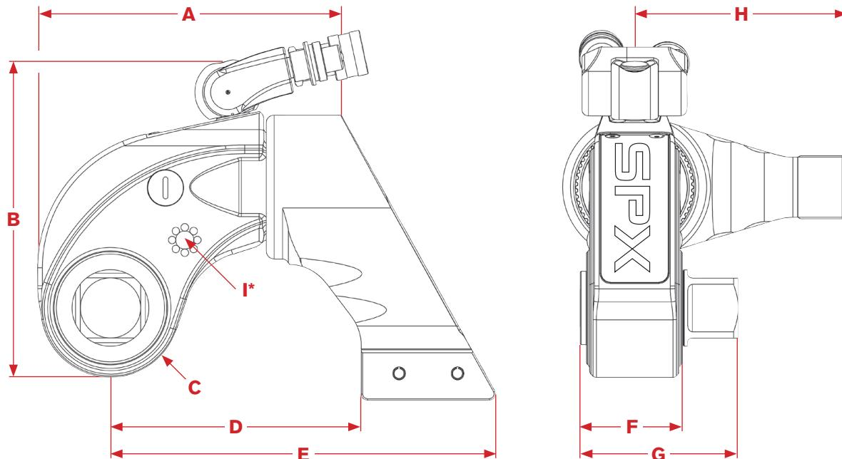
\* Dimension I shows thread size (on both sides of the tool) for safety handle or lifting point.
