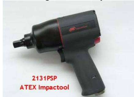
low spark body and the high efficiency twin hammer impact mechanism it delivers a maximum of 816 Nm of torque from a package weighing less than 2kg. Compare that with any of the competitor’s offerings!
