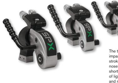
The tool's designed long-stroke mechanism imparts a minimum 30 degree nut rotation per stroke while maintaining a tight and compact nose radius: this is a clear advantage over the short stroke and back-up pawl mechanisms of light alloy competitive models. Fewer parts and reduced torsion in operation - equals reduced wear, maintenance and associated costs.
