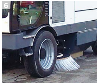
6 Third side brush can work on both sides of the machine. Joystick-driven by the operator.
