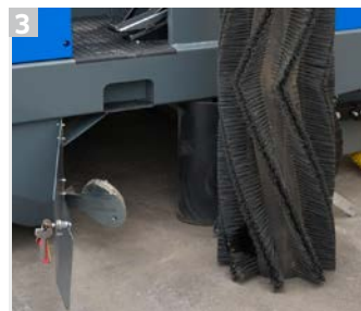
3 Main brush can be replaced easily without tools.
