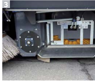
3 Patented CDS clever detective system to control and adjust the pressure on central broom. Useful to sweep on bollard speed and uneven ground.
