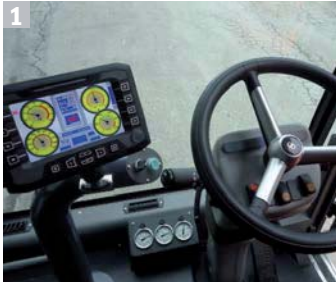
1 Control Panel. Touchscreen dashboard with Can Bus system.
