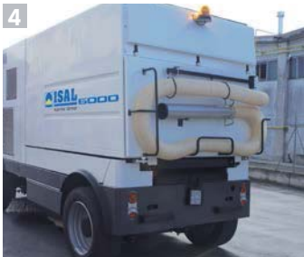
4 Wander hose to suck debris. For complete cleaning of areas not easily reachable by the machine.
