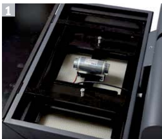
1 Horizontal flat filter system. Polyester panel filter with electric filter shaker. 6 m 2 filter surface area.
