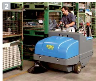
1 Horizontal flat filter system. Polyester panel filter with electric filter shaker. 6 m 2 filter surface area.
